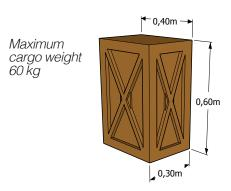
In the cabin seats max. 18 packages, size 60x40x30 cm and indicative weight limit 60 kg/package. In addition, cargo space carries 245 kg.
