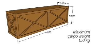
On the cargo stretcher in the cabin. Maximum weight limit is 150 kg and maximum container measurements 200x52x60 cm. In addition, the aircraft fits six passengers or six parcels of 60x40x30 cm and 60 kg each. In addition, cargo space carries 245 kg.
